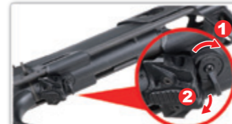
Turn the stock catch knob clockwise, then flip up the stock release button set to remove the stock.
